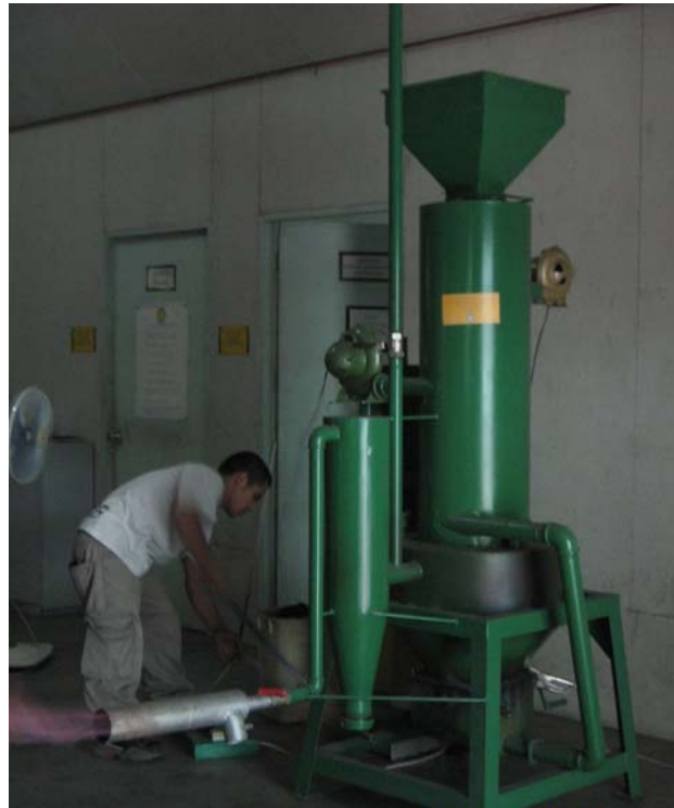
Pictorial of the Continuous-Flow Rice Husk Gasifier
