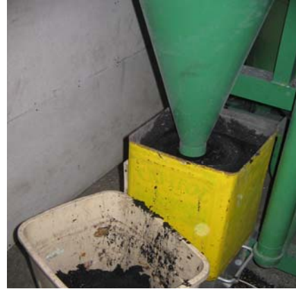
Sample of Char Coming Out from the Gasifier
