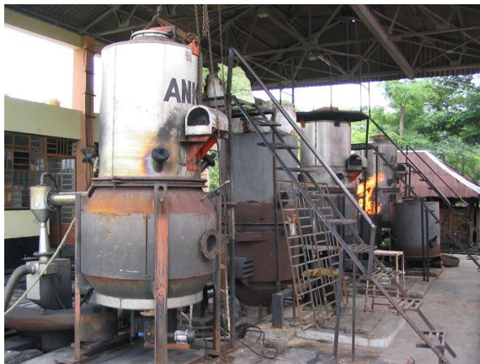
Figure 2. 5 x 100 kW biomass gasifier at Gosaba Rural Energy Cooperative, West Bengal State
